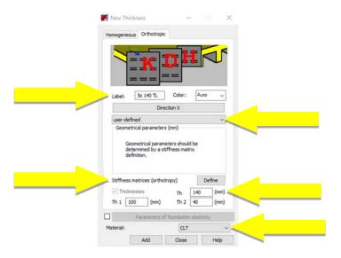
**Note:** The thicknesses "Th", "Th1" and "Th2" (total and sums of in x- and y-direction) have to be added manually. They do not influence the results, if the correct stiffness parameters are given (see step 2d).
