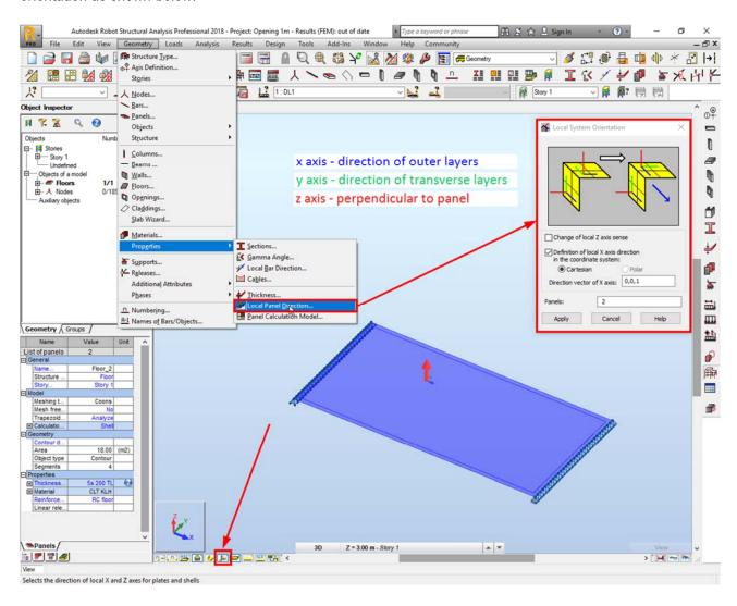
Note: The local x-direction of the panel is always the direction of outer layers (according to the definitions in KLHdesigner).
