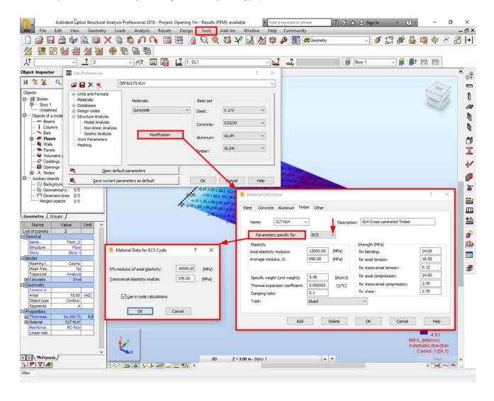
**Note:** The material values you aplly here do not influence the results as long as the stiffness parameters are given correctly. The Specific weight will be used to calculate the self weight of the structure (in combination with the total thickness "Th").
